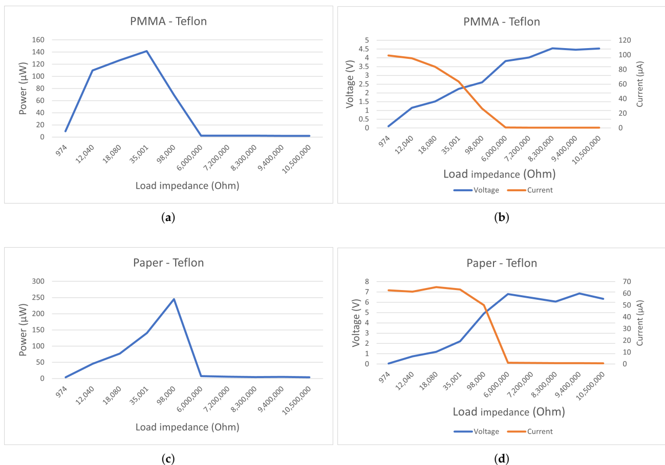
Figure 17. Converted power versus load resistance from PMMA-Teflon (a); Output current/voltage for different loads from PMMA-Teflon (b); Converted power versus load resistance from Paper-Teflon (c); Output current/voltage for different loads from PMMA-Teflon (d).
