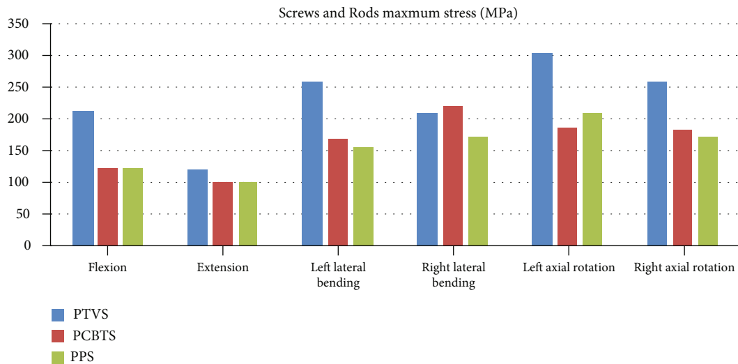
FIGURE 10: Screws and rods maximum stress (MPa) (blue column: PTVS; red column: PCBTS; green column: PPS).
