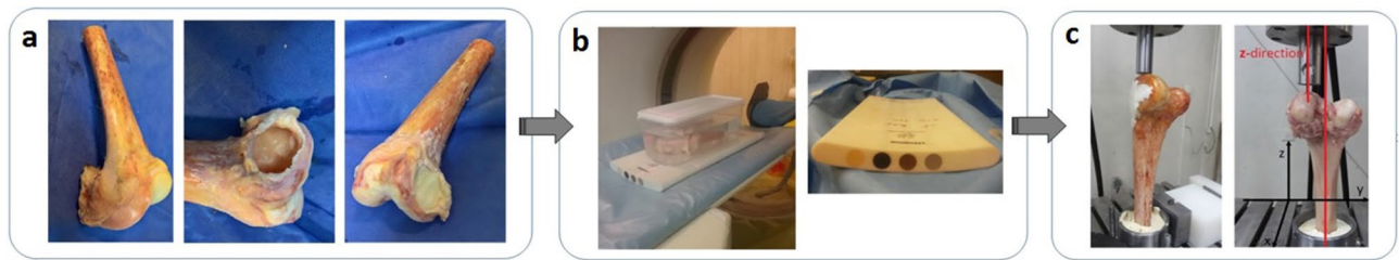
Figure 1. Various experimental phases of this study: (a) Specimen preparation, tumour surgery was mimicked in one sample of each pair while the contralateral femur remained intact; (b) QCT scan and the calibration phantom; and (c) Mechanical tests of a defective and an intact specimen. The compressive load was applied in the z-direction, parallel to the bone shaft.
