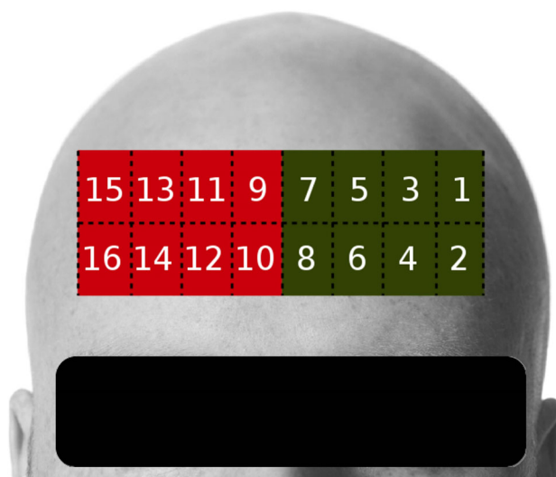
Fig. 1 Voxel distribution of device containing 16 voxels. The voxels can be grouped into those corresponding to brain's left hemisphere (green) and right hemisphere (red)
