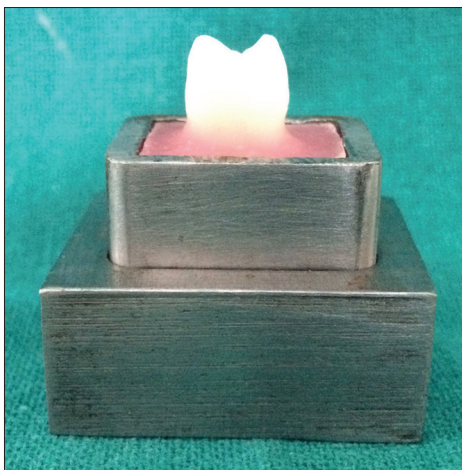
Figure 1: Mounted specimen in custom made metallic mold
