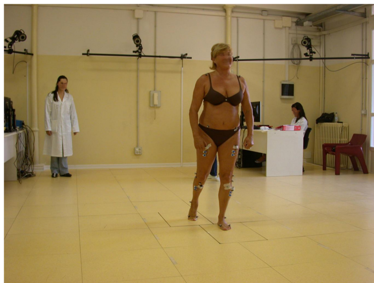
Figure 7 Standard gait analysis. A picture taken in the gait analysis laboratory of the authors during data collection for level walking; a patient implanted with TAR is shown. The marker-set is typical of a pelvis plus lower limb motion analysis according to Leardini et al. [38], with three markers only on the foot, considered as a single rigid body, as well as the shank, thigh and pelvis.
