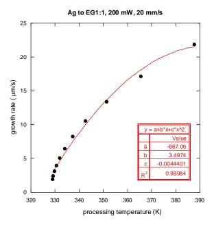
**Figure 9.** Variation of the silver line growth rate (in thickness) with respect to the processing temperature. The filled dots: the filled dots shown here were obtained using the fitted curve in Figure 7a.
