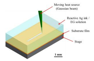
Figure 3. A schematic of the simulation domain used in the current study.
