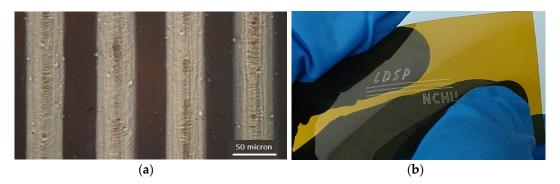
**Figure 6.** Silver lines fabricated on polyimide film substrate using LDSP (with ethylene glycol (EG) based solution): (a) microscopic picture of the silver line; (b) a demonstration of silver patterns on the flexible PI substrate.
