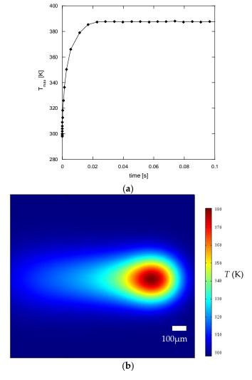
**Figure 8.** (a) The processing temperature for the first scan with respect to time along the scan path; (b) The simulated temperature profile on the polyimide surface.
