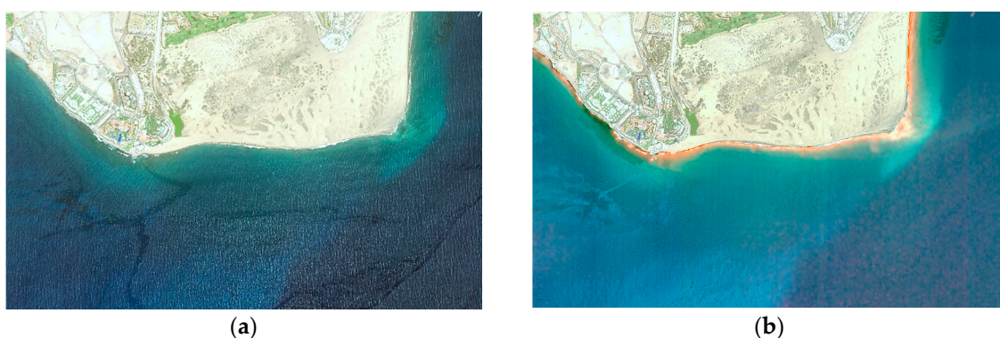
Figure 4. (a) WorldView-2 color composite image of Maspalomas (Gran Canaria Island, June 2015) and (b) image after sunlint correction using the algorithm implemented in [28].
