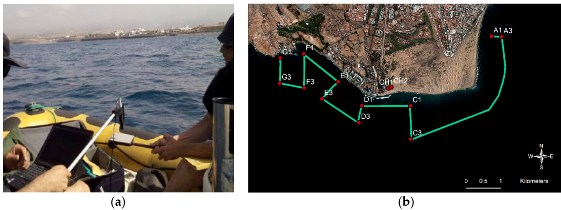
Figure 2. (a) Procedure of ground-based spectral data acquisition with the ADS Fieldspec 3 and; (b) ship transects and sampling sites during the Maspalomas field campaign of June 2015.
