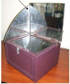
Figure 1. Box type solar cooker used in this study (A) original design (left) with control box (right) and (B) final design with additional reflector. doi:10.1371/journal.pone.0001100.q001
