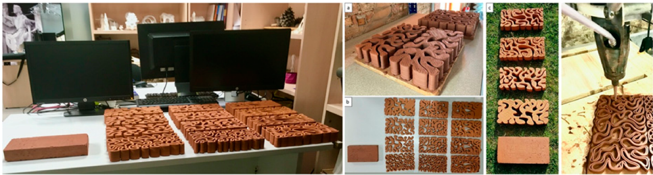
Figure 10. Alberto T. Estévez (Yomna K. Abdallah, computational designer), Biodigital Barcelona Bricks (3D-printed clay), GENARQ/iBAG, UIC Barcelona. (a–c) show different iterations (V1, V2, and V3) printed with clay. Right: 3D printing process of the linear model. Photos by the author.
