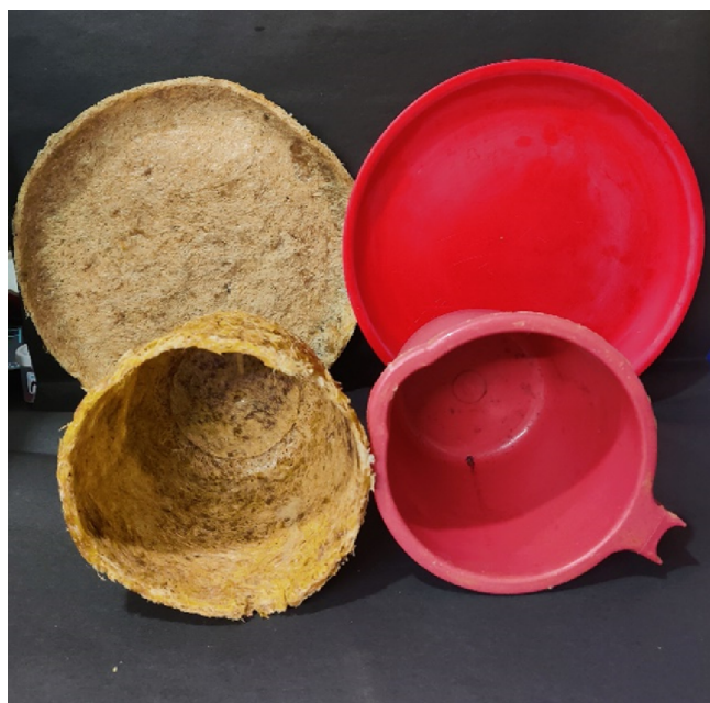
Figure 10. Plate and pot developed using treated waste filature silk-wheat gluten composite sheets representing the feasibility of preparing various biodegradable products.
