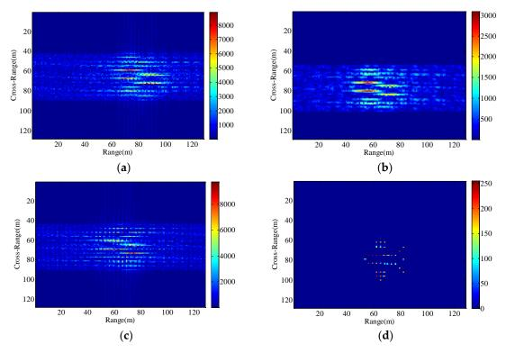
**Figure 11.** Imaging results with the radar platform vibration parameters P6. (a) RD algorithm; (b) cross-correlation method; (c) minimum entropy method; (d) the proposed method.
