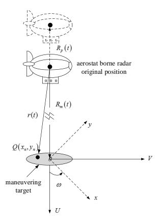
Figure 1. Aerostat borne ISAR imaging geometry model.
