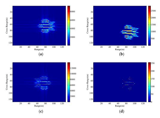
**Figure 10.** Imaging results with the radar platform vibration parameters P5. (a) RD algorithm; (b) cross-correlation method; (c) minimum entropy method; (d) the proposed method.
