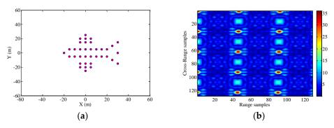
**Figure 4.** (a) A hypothetical target composed of perfect point scatterers. (b) The amplitude of the raw data.
