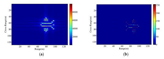
**Figure 5.** Imaging results with the radar platform displacement parameters P1. (a) RD algorithm; (b) the proposed method.
