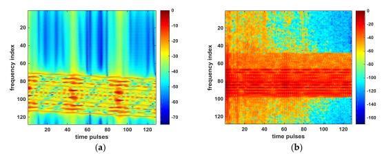
**Figure 9.** Spectrograms of time pulses. (a) before applying the proposed method; (b) after applying the proposed method.
