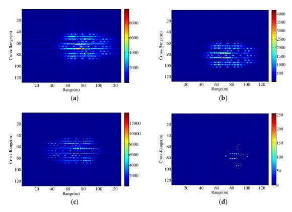
**Figure 12.** Imaging results with the radar platform vibration parameters P7. (a) RD algorithm; (b) cross-correlation method; (c) minimum entropy method; (d) the proposed method.
