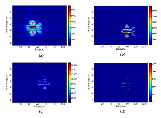
**Figure 6.** Imaging results with the radar platform displacement parameters P2. (a) RD algorithm; (b) cross-correlation method; (c) minimum entropy method; (d) the proposed method.
