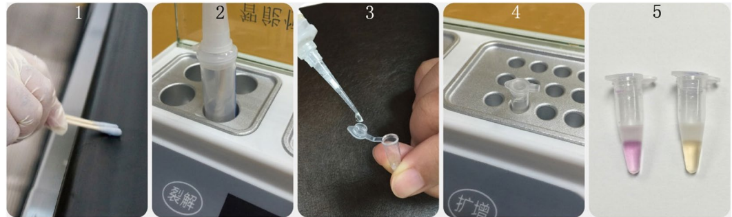
Figure 9. Operational steps of the novel kit for rapid nucleic acid test in field settings. 1. Use cotton swabs for sampling. 2. Heat the tube for DNA denaturation. 3. Squeeze out two droplets. 4. Amplify the DNA at a constant temperature. 5. Observe the results.
