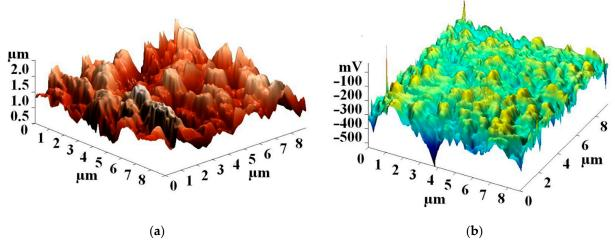
Figure 5. Topology (a) and distribution of the surface potential (b) of the aligned multi-walled CNTs combined into bundles.
