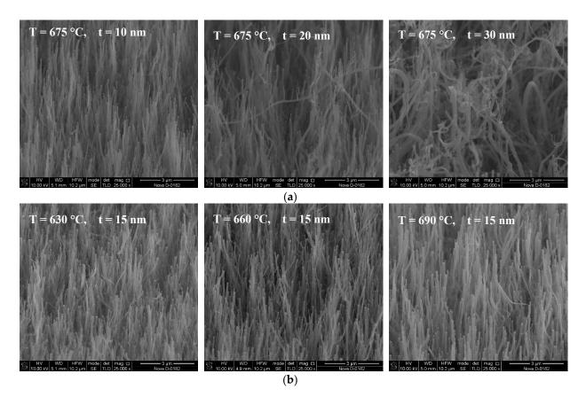
**Figure 1.** (a) SEM images of CNT arrays grown at a temperature of 675  $^{\circ}$ C and a catalytic layer thickness *t* ranging from 10 to 30 nm, and (b) at a catalytic layer thickness of 15 nm and an increase in temperature from 660 to 690  $^{\circ}$ C.
