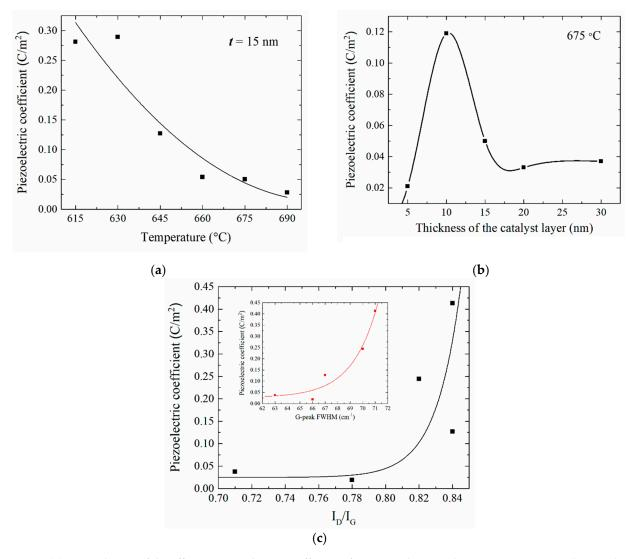
**Figure 7.** (a) Dependences of the effective piezoelectric coefficient of CNTs on the growth temperature at a catalytic Ni layer of 15 nm, (b) on the thickness of the catalytic Ni layer at a temperature of 675 °C and (c) on the defectiveness of CNTs. The inset in Figure 5c shows the dependence of the piezoelectric coefficient of CNTs on the full width at half maximum of the G-peak of the CNT spectra, reflecting the change in the curvature of the surface of the graphene sheet forming the CNT.
