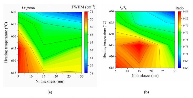
**Figure 3.** Maps of the FWHM distribution of the G-peak (**a**) and the ratio of the intensities of the D- and G- peaks  $I_D / I_G$  (**b**) of the Raman spectra of CNT arrays versus the growth temperature and the thickness of the catalytic layer.
