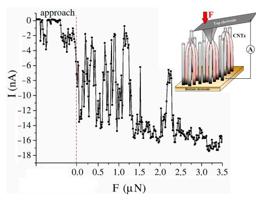
**Figure 6.** Dependence of the current generated during the deformation of CNTs grown at a temperature of 615 °C and a catalytic nickel layer thickness of 15 nm on the pressing force of the AFM probe to the CNT array surface. The inset shows a schematic representation of the measurement process.
