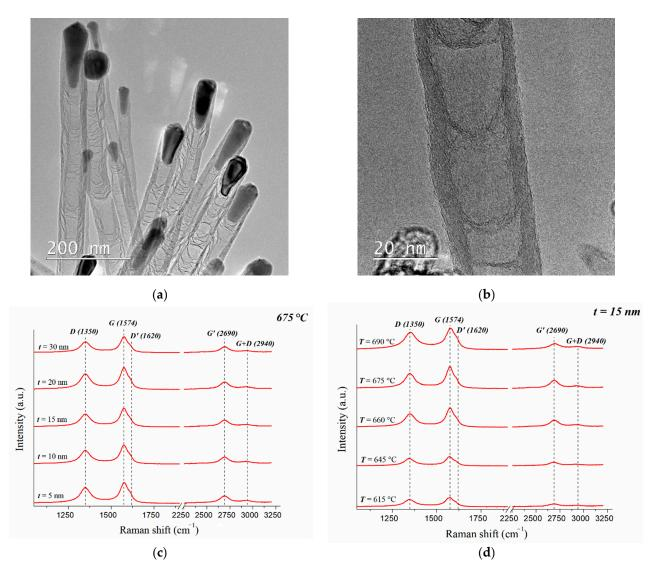
**Figure 2.** TEM images of the studied CNTs (**a**,**b**). Raman spectra of CNT arrays grown at a temperature of 675 °C and a catalytic layer thickness of 5 to 30 nm (**c**), and at a catalytic layer thickness of 15 nm with an increase in temperature from 615 to 690 °C (**d**).
