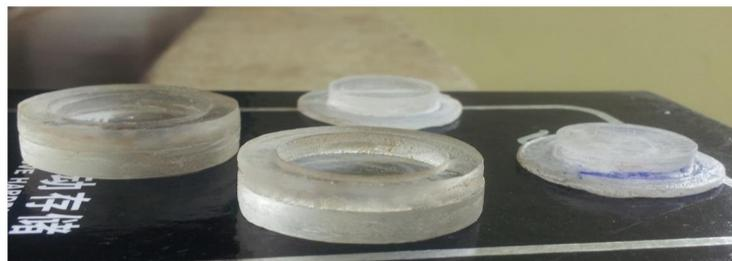
**Fig 1. Encapsulation cup used for holding the films for radiation dosimetry.** The films were positioned at  $D_{max}$ . The cup was constructed with Perspex and had a dimension of 4 cm (cross-sectional diameter) x 1 cm (thickness).
