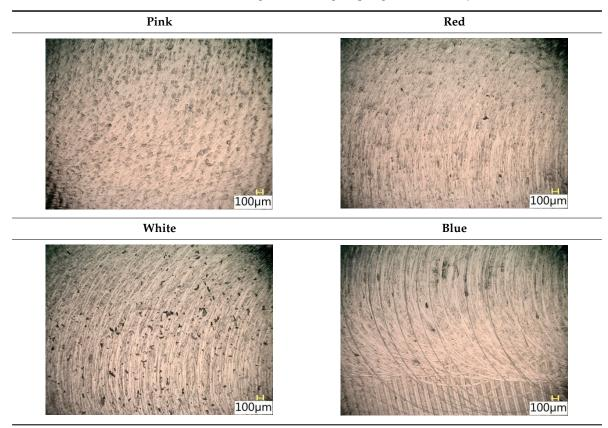
Table 6. Surface texture after brushing with the "high" spring in the offset adjustment sleeve.
