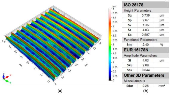
Figure 12. Roughness following milling: (a) topography; (b) parameters.
