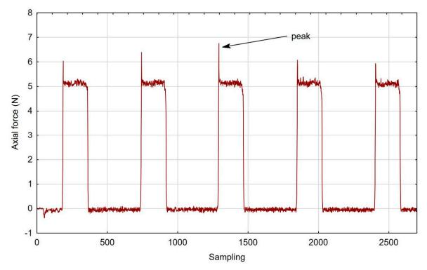
**Figure 7.** Axial force during brush treatment with the white fibre tool and "low" spring in the offset adjustment sleeve.
