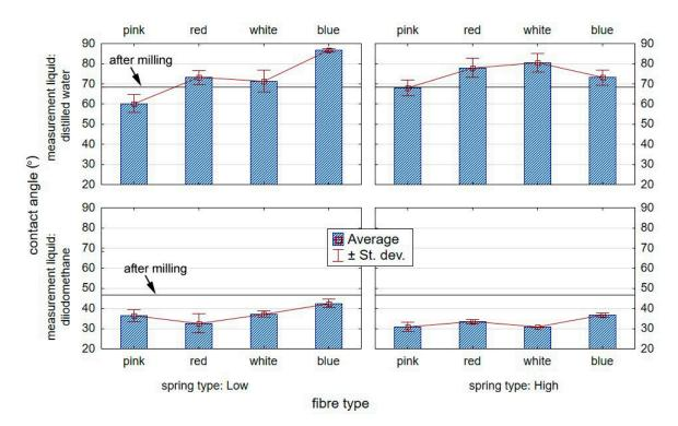
Figure 14. Effect of brushing on the value of the contact angle on the surface of an aluminium alloy.
