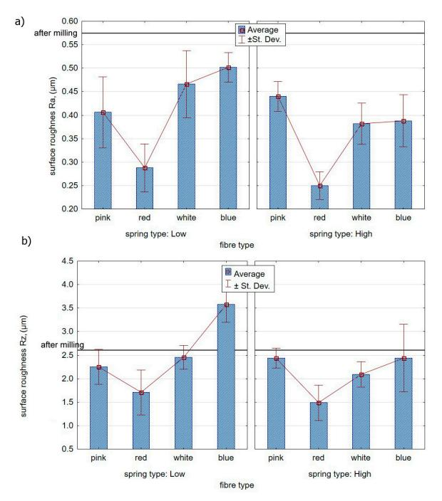
**Figure 11.** Effect of the fibre type and spring in the offset adjustment sleeve on the surface roughness: (a) Ra parameter; (b) Rz parameter.
