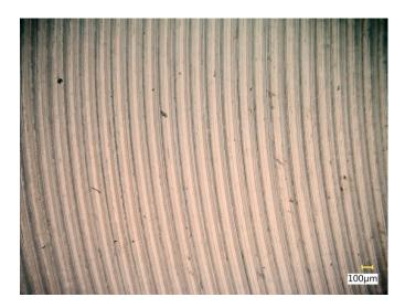
Figure 13. View of the surface after milling.
