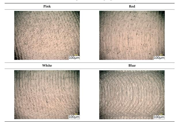
Table 5. Surface texture after brushing with the "low" spring in the offset adjustment sleeve.
