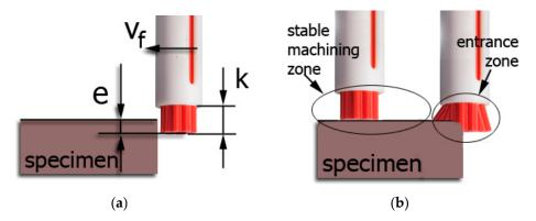
**Figure 4.** Brushing process: (**a**) graphical representation of infeed "e" and fibre projection length from sleeve "k"; (**b**) machining zone presentation.
