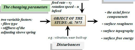
Figure 2. Schematic diagram of the study object.
