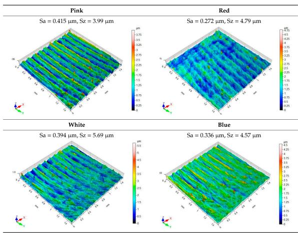
Table 4 presents sample maps showing the surface topography after brushing treatment for the "high" spring in the adjustment sleeve. In the case of fibres with higher stiffness (i.e., white and blue), characteristic scratches are clearly visible on the roughness maps which are the result of more aggressive subtraction of material by the brush fibres, compared to softer fibres (i.e., pink and red). The effect was further confirmed by the increase in the values of the Rz parameter.
