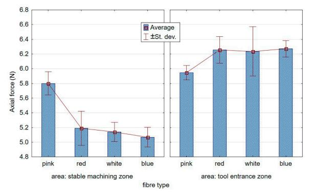
**Figure 8.** Effect of the fibre type on axial forces at the tool entrance zone and the stable course for the "low" spring in the offset adjustment sleeve.
