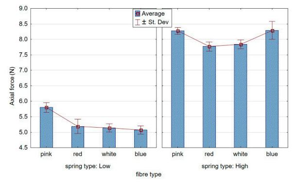
Figure 10. Effect of the fibre type on the axial force in the stable cutting zone for the two tested springs.
