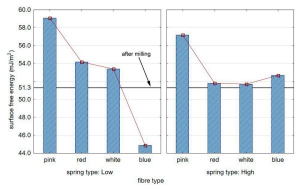
Figure 15. The impact of the brush type on the SFE (surface free energy) of the aluminium alloys.
