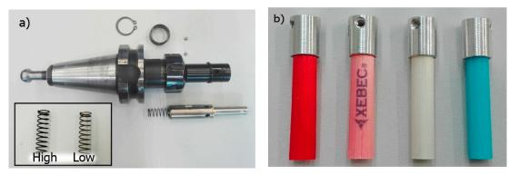
Figure 3. Ceramic brushes: (a) brush adjustment sleeve; (b) fibre types.
