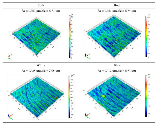
Table 4. Surface topography after brushing with the "high" spring in the offset adjustment sleeve.
