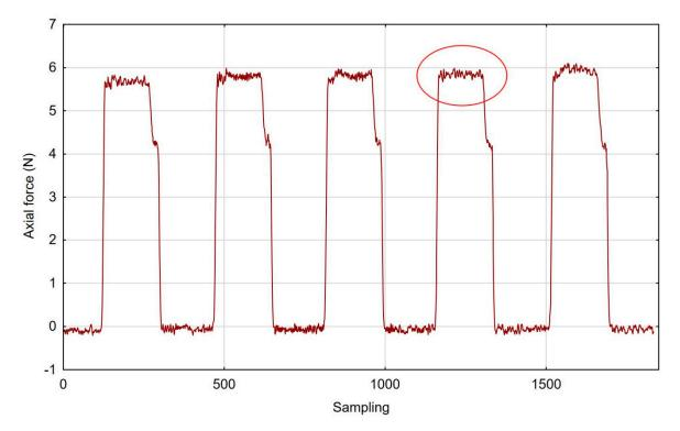
**Figure 6.** Axial force during brush treatment with the pink fibre tool and "low" spring in the offset adjustment sleeve.
