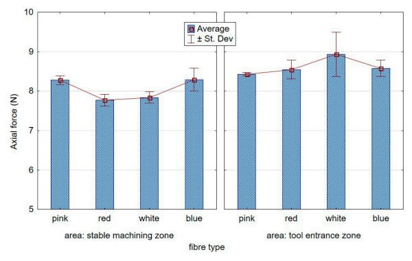
**Figure 9.** Effect of the fibre type on the axial forces at the tool entrance zone and the stable course for the "high" spring in the offset adjustment sleeve.
