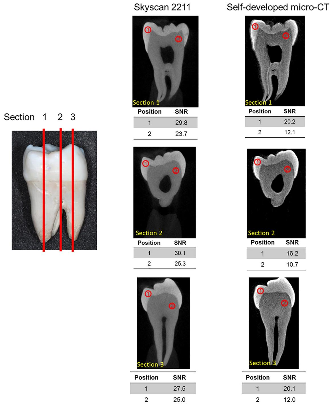
**Fig 4.** Quantitative analysis of the three buccal-lingual reconstructed images of the third molar captured with (left) the Skyscan 2211 and (right) the self-assembled micro-CT system. SNR, signal-to-noise ratio.
