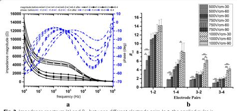
**Fig. 3** Impedance spectrum (**a**) and  $R_{\text{rel}}$  between different electrode pairs. In **a**, the applied pulse is with group 4 parameters (pulse amplitude: 750 V, pulse number: 30) in Table 1. In **b**, 500 V-30 means the magnitude of the electric field is 500 V and the pulse number is 30 (group 1 in Table 1). (\*\*p < 0.01, \*p < 0.05)
