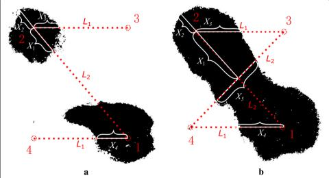
**Fig. 2** Sketch of the square edge, diagonal and length of the ablation area in different directions. **a** Ablation zone is not connected—treated by 30, 500 V pulses (group 1). **b** Ablation zone is connected—treated by 90, 500 V pulses (group 3)
