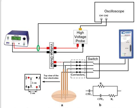
**Fig. 1** Schematic of the experimental setup (**a**) and the equivalent circuit model (**b**). The dashed line in (**a**) indicates that these two lines are shared with the two lines connected to Gamry, and the four connectors should be disconnected when applying high voltage pulses. The shadow in the potato is the mid-plane of the ablation zone that was cut
