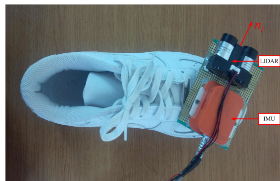
Figure 6. IMU and LIDAR system for the experiment.
