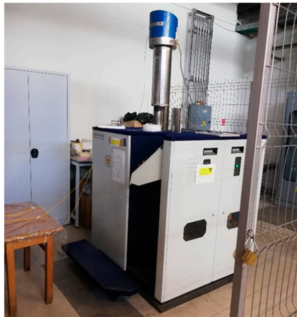
Figure 3. Photo of the irradiation and measurement setup based on the GC-5000.
