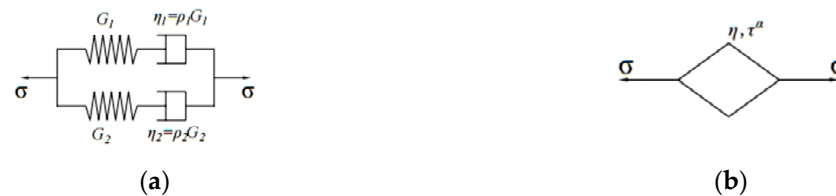
Figure 7. Relaxation modulus fitting model: (a) The second-order extensive Maxwell model; (b) the Scott-Blair model.
