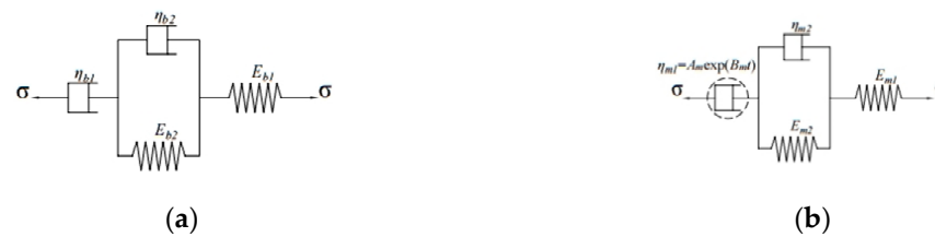
Figure 3. Creep compliance fitting model: (a) the Burgers model; (b) the modified Burgers model.
