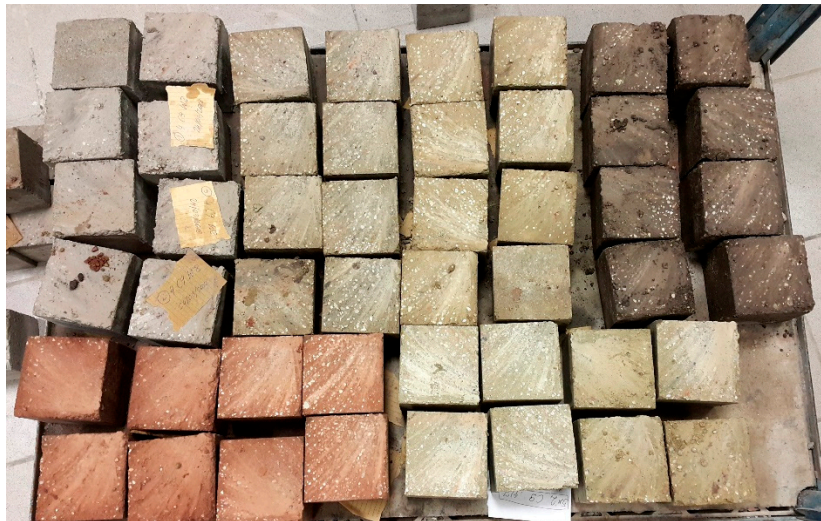
Figure 6. Part of the CSRE samples on which the compressive strength tests were made.
