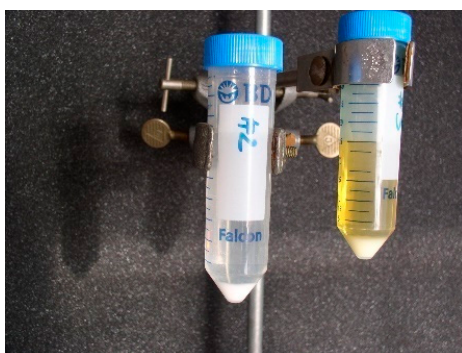
Figure 4. Dissolving ceramics in an acid medium HNO 3 +HF.
