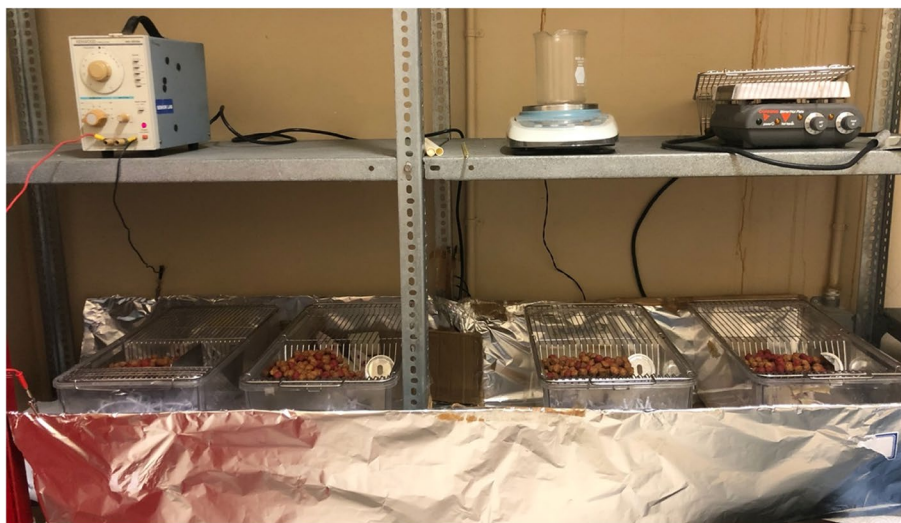
Fig. 1 Experiment Set-up showing EMR source used to create an electric field for the experimental group
