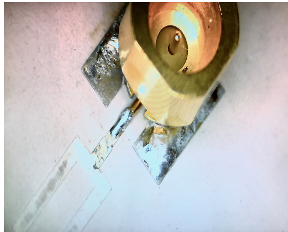
Figure 4. Mounted SMPM connector on the ground pad of the antenna element.
