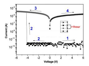
**Figure 5.** Current-voltage (I–V) characteristics of the ITO/polymer/Al memory device as a representative of WORM characteristic. (The third sweep was conducted more than one hour after turning off the power).
