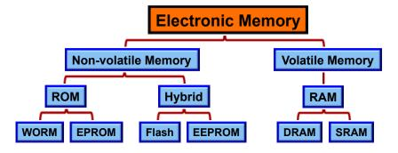
Figure 1. Classification of electronic memories. ROM: read-only memory; RAM: random-access memory; EPROM: erasable programmable read-only memory; EEPROM: electrically erasable programmable read-only memory.
