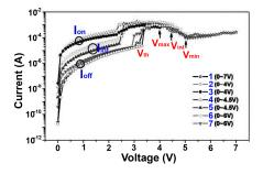
**Figure 6.** Current-voltage (I–V) characteristics of the ITO/polymer/Al memory device as a representative of NDR characteristic.
