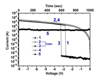
**Figure 2.** Current-voltage (I–V) characteristics of the indium tin oxide (ITO)/polymer/Al memory device as a representative of DRAM characteristic. (The third sweep was conducted about 1 min after turning off the power).
