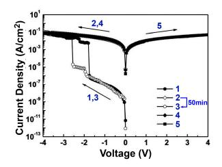
**Figure 3.** Current-voltage (I–V) characteristics of the ITO/polymer/Al memory device as a representative of SRAM characteristic. (The third sweep was conducted about 50 min after turning off the power).
