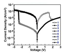
**Figure 4.** Current-voltage (I–V) characteristics of the ITO/polymer/Al memory device as a representative of Flash characteristic.
