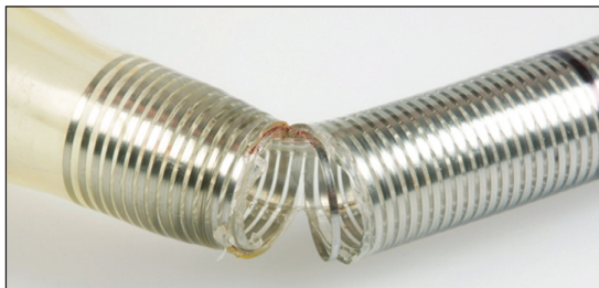
Figure 11 - Fracture of a double-lumen venous cannula (Avalon®)
