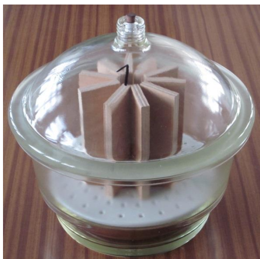
Figure 1. Plywood samples in the glass desiccator.
