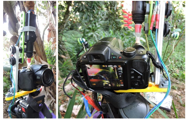
FIGURE 4 Photographs of the system deployed in the field. The left photograph shows the mounting of the actuator positioned to press the camera's shutter. Our mount used Meccano™ pieces (Meccano S.N., Calais, France), although simple hardware or an articulating arm would suffice. On the right the camera is shown in prerecord mode with two PIR sensors in the background. Camera standby time was extended using an external AA battery pack connected to the camera's power socket (blue and red wires). The trigger box (not visible) is below the camera
