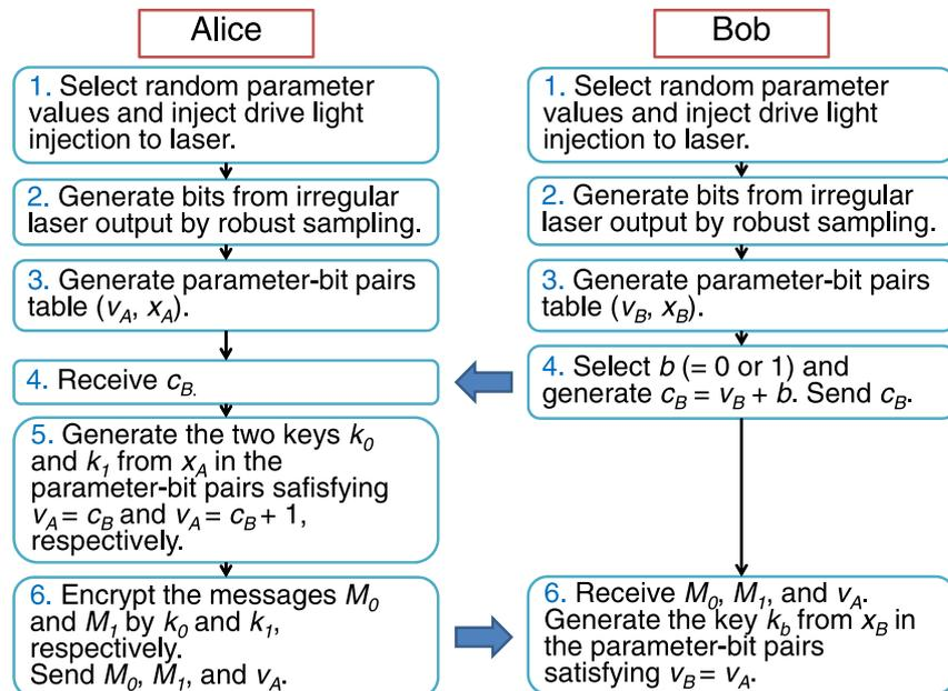
**Figure 2.** Protocol of one-out-of-two oblivious transfer. + Denotes bitwise exclusive-OR operation.  $v_{A,B}$ : random observation parameters for Alice and Bob.  $x_{A,B}$ : observed bits for Alice and Bob.
