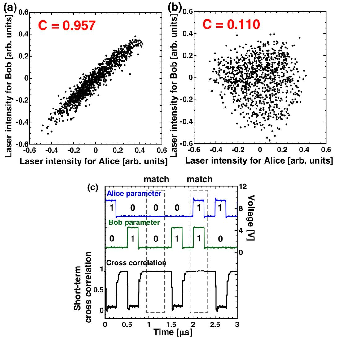
**Figure 3.** Experimental result of optical correlated randomness. (a,b) Correlation plots of temporal waveforms of Alice's and Bob's laser outputs.  $C$  indicates cross-correlation value. (a) Same parameter selection, and (b) different parameter selection. (c) Example of parameter switching. Alice's and Bob's parameter values and the short-term cross-correlation between Alice's and Bob's temporal waveforms are shown.
