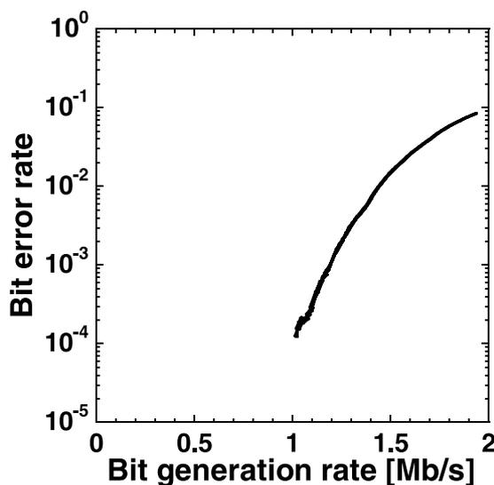
**Figure 4.** Relation between bit error rate (BER) and bit generation rate (BGR) for parameter-bit observation pairs of optical correlated random source for oblivious transfer. The two threshold values of the robust sampling are changed.
