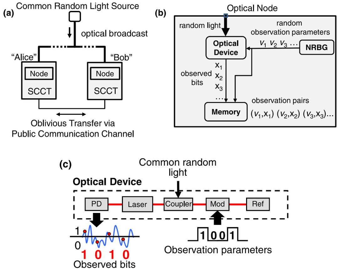
**Figure 1.** Schematic diagram of system for oblivious transfer using optical correlated randomness. (a) Total system, (b) optical node, and (c) optical device. (a) SCCT: secure communication and computation terminal. (b) NRBG: non-deterministic random bit generator. (c) Mod: optical phase modulator, PD: photodetector, and Ref: optical reflector.
