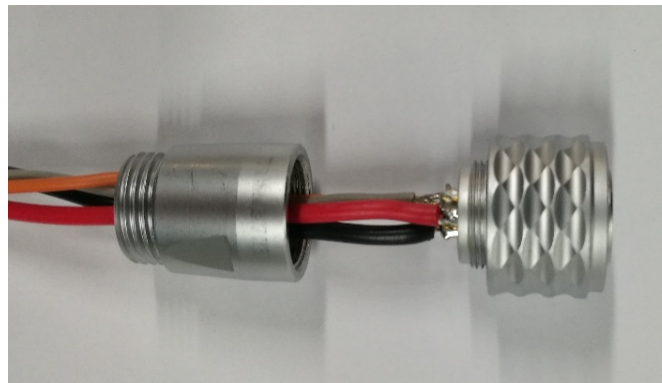
Figure 26. Pin circuit welding of aviation plug.
