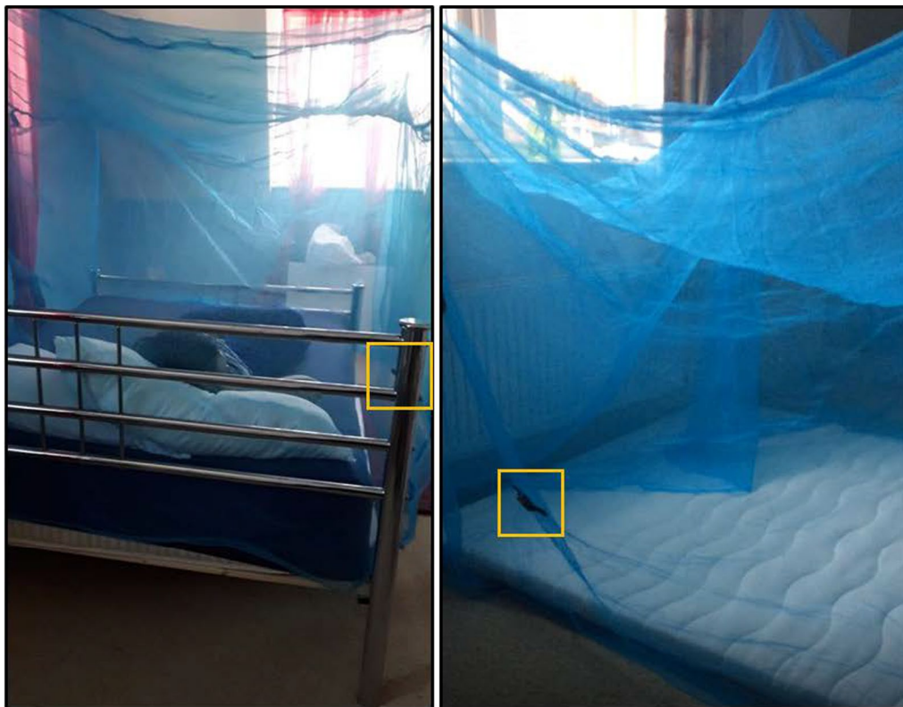
Fig. 1 Photographs of accelerometer and placement when fixed on bed nets. Boxes identify where on the bed nets the accelerometers were fixed. In the photograph on the left, the device is visible just behind the bed post
