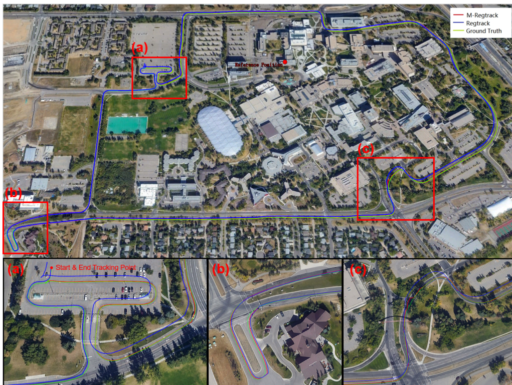
Figure 13. The ground truth map and the tracking result comparison of different methods for the moving car experiment Section 3.2.3, where the red dot was the reference receiver, the (a–c) indicate the enlarged parts.
