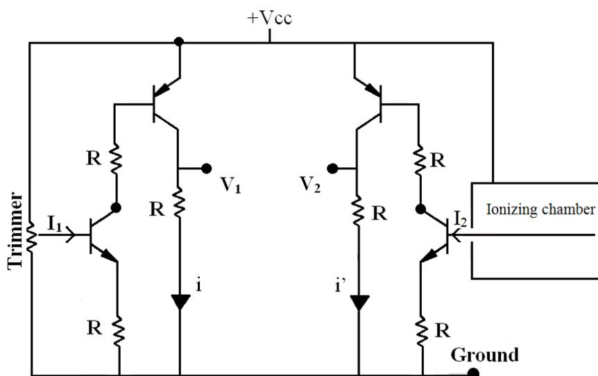
**Figure 4:** Two npn and two pnp Darlington Transistors are connected to the ionization chamber consisting of an anode (a needle passing through the canister) and a cylindrical cathode (the canister).
