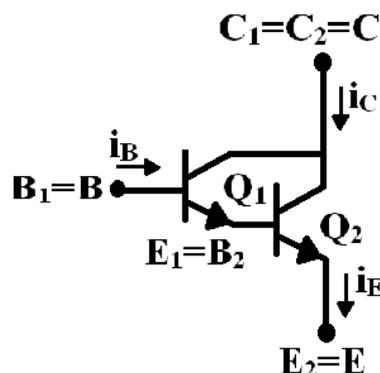
**Figure 1:** Two single transistors ( $Q_1$  and  $Q_2$ ) are combined to form Darlington Transistors
