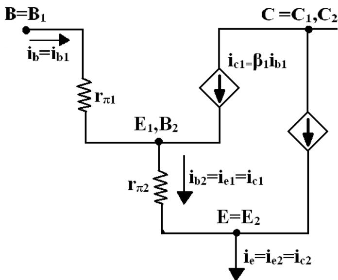
Figure 2: Two npn BJTs which are cascaded behave like a single npn transistor
