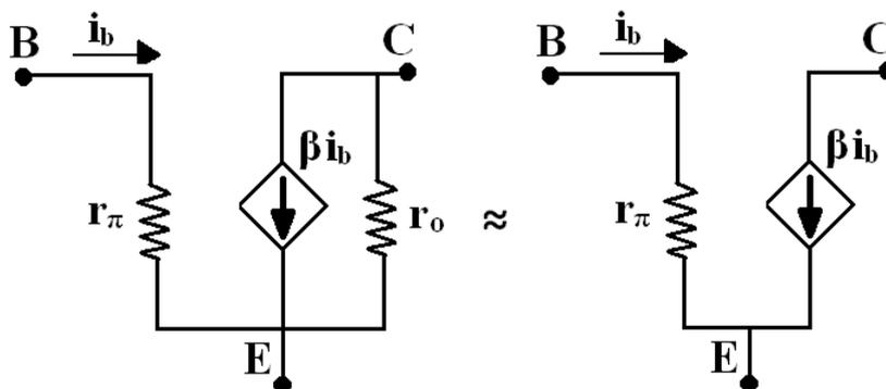
Figure 3: The ac small signal model of the npn version of each transistor
