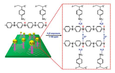
**Figure 3.** Possible mechanism for molecular interactions between the PSS-doped PANI/graphene nanocomposites and H<sub>2</sub>S gas molecules. Reproduced from [64], with permission from the Royal Society of Chemistry.
