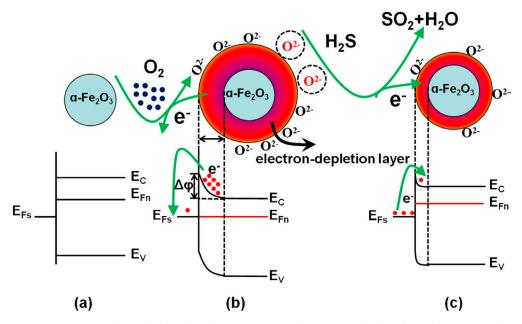
$E_C$ : bottom of conduction band;  $E_V$ : top of valence band;  $E_{Fn}$ : bulk Fermi level;  $E_{Fs}$ : surface Fermi level;  $\Delta \phi$ : potential barrier
