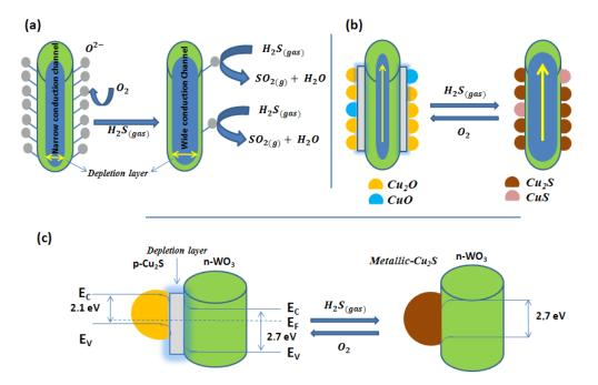
**Figure 2.**  $H_2S$  gas sensing mechanism of (a) pure  $WO_3$  nanowires, (b)  $Cu_2O/CuO$  nanoparticle-functionalized  $WO_3$  nanowires, and (c) an example of the evolution of the  $Cu_2O$  nanoparticle/ $WO_3$  nanowire p-n heterojunction before and after exposure to  $H_2S$ . Reproduced from [47], with permission from the American Chemical Society.
