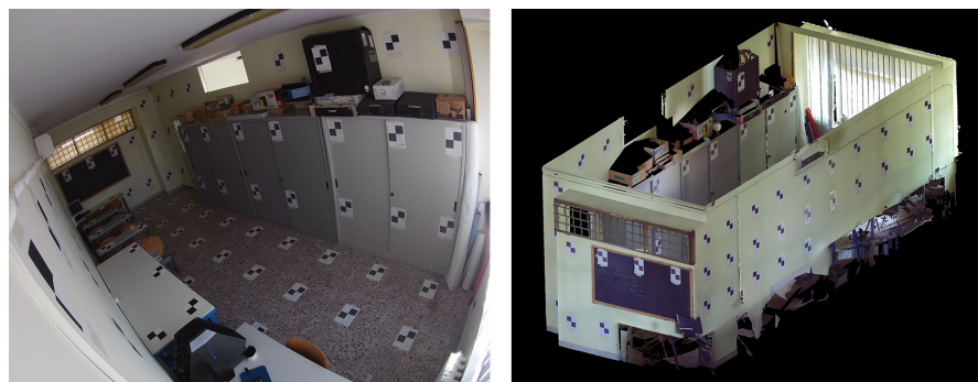
FIGURE 5 Test field with 92 target (left), Point Cloud (right) [Color figure can be viewed at wileyonlinelibrary.com ]
