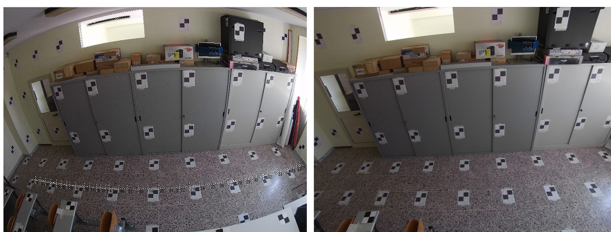
FIGURE 11 The line used in Amped FIVE to calibrate the camera and the distortion-free image produced by Amped FIVE [Color figure can be viewed at wileyonlinelibrary.com ]
