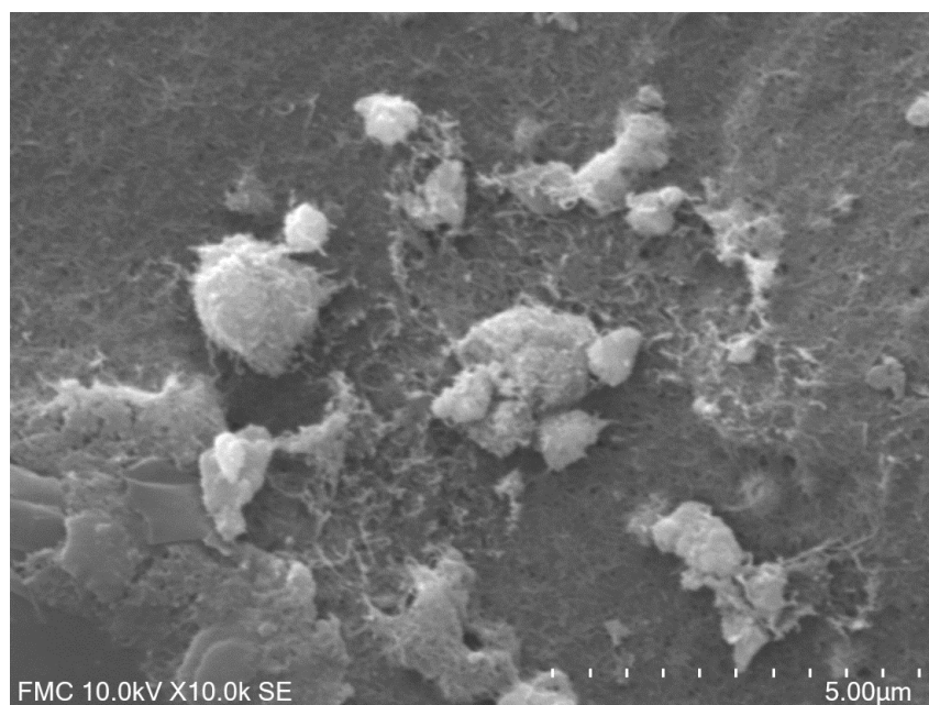
Figure 1. Scanning electron microscope (SEM) image of CSPE modified with tyrosinase/platinum nanoparticles/graphene/chitosan (Ty/PtNP/GPH/Chit) bionanocomposite.
