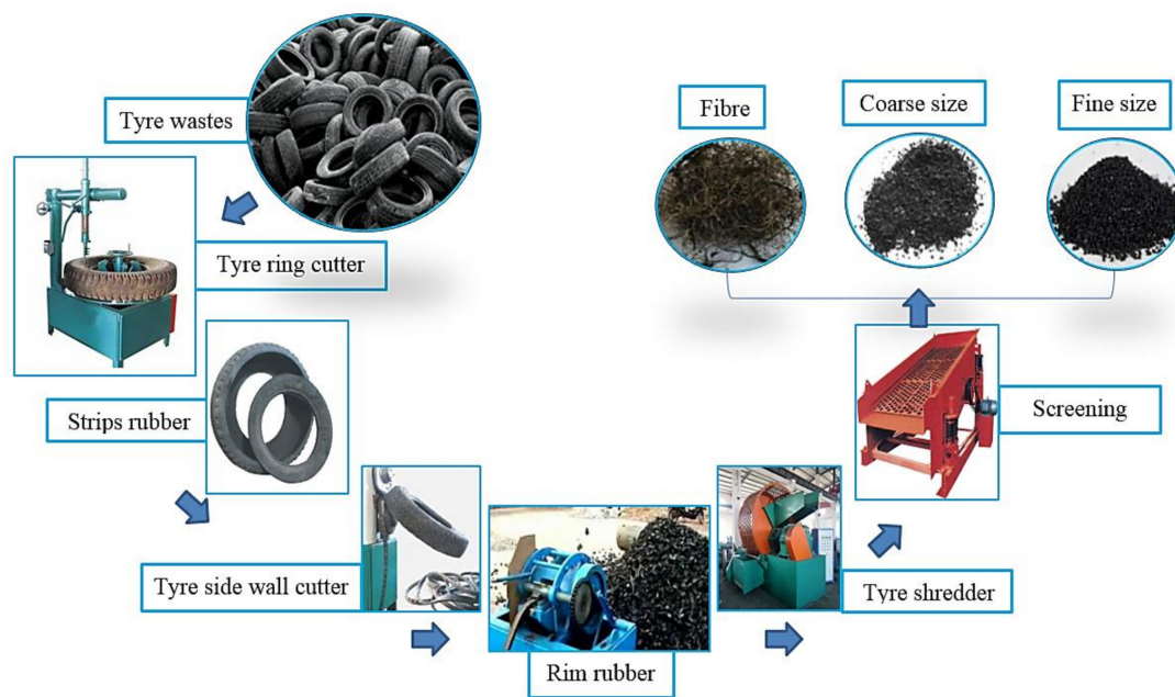
Figure 1. Fine and coarse waste rubber tire crumbs (WRTCs) preparation process.
