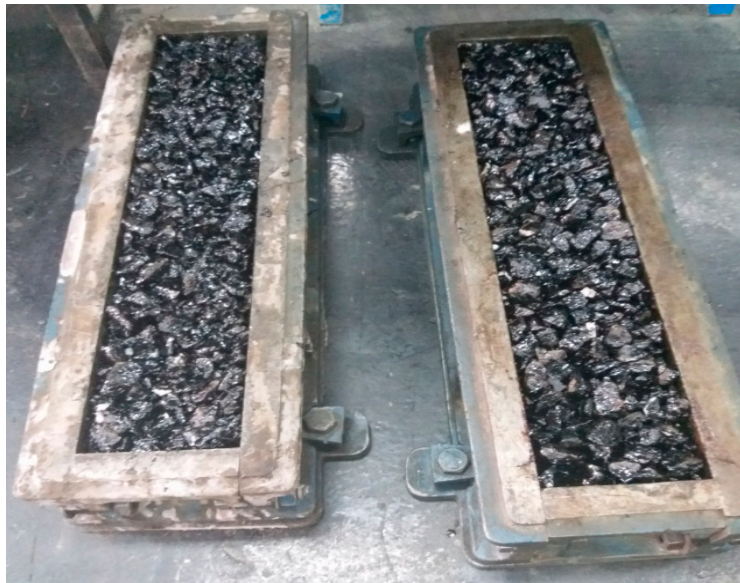
Figure 2. Beam samples of porous asphalt mixtures for flexural test.
