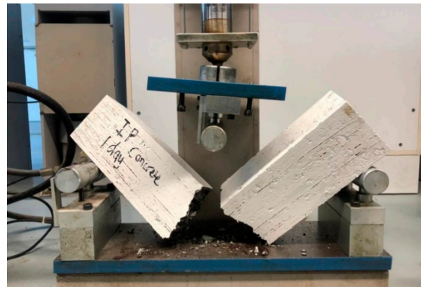
Figure 4. Experimental test to measure flexural strength of semi-flexible beam.
