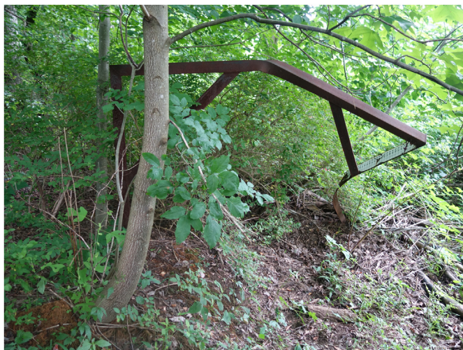
Figure 3. Steel stream staffplate twisted and damaged by debris impacts, probably during the 1977 flood. The staffplate now resides on the floodplain within the breach of the South Fork Dam at Johnstown Flood National Memorial (image credit: C. Coughenour).
