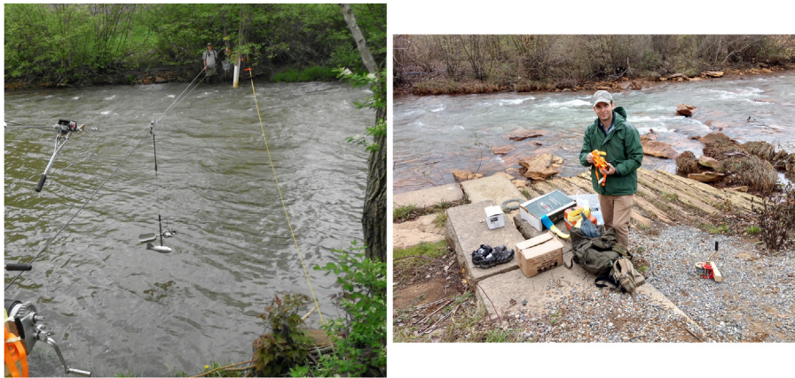
Figure 7. Left: Cableway discharge measurement at the gaging station on the South Fork of the Little Conemaugh River in Johnstown Flood National Memorial. Just to the right of the photo lies the corner foundation stone of the former control tower of the South Fork Dam. Right: Just upstream of the gage with visible foundation elements. A lower dressed stone just behind that where the equipment is resting was previously surveyed at elevation of 1,544.93 ft.
