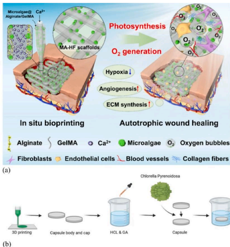
Fig. 6. (a) In situ 3D bioprinting of live photosynthetic scaffolds for autotrophic wound healing (Wang et al., 2022); (b) preparation process of 3D-printed cylindrical capsule structure and schematic of immobilized C. pyrenoidosa adsorption experiment.
