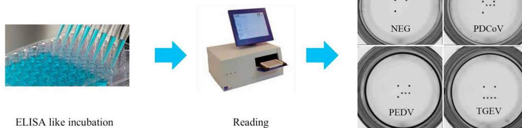
Fig. 1. Overview of the design, fabrication and use of the AgroDiag porcine enteric coronavirus (PEC) multiplex planar immunoassay. (A) Manufacturing steps include functionalization of the wells of a microplate with a dextran layer before printing of the protein array in triplicate. (B) The assay protocol and working principle is similar to the solid-phase standard indirect ELISA. After the three typical incubation steps (serum sample, conjugate, and substrate), followed by microplate reading. The reaction was visualized as brown spots which intensity correlated with antibody levels to specific viral antigen target in the array. Four results are obtainable depending on incubation with a negative control, or samples from PDCoV, PEDV, TGEV inoculation groups. Scale bar corresponds to 1 mm. (For interpretation of the references to colour in this figure legend, the reader is referred to the web version of this article.)
