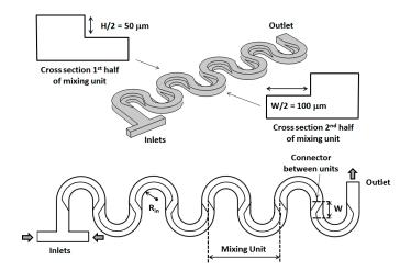
**Figure 2.** 3D and top views of the new serpentine micromixer design employing non-rectangular cross-sections. As shown above, the orientation of the cross-section of the mixer is changed after each turn of the serpentine.
