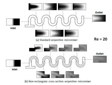
**Figure 5.** Transversal concentration distribution at various positions along the channel for (**a**) a standard serpentine micromixer and (**b**) a serpentine micromixer with a non-rectangular cross-section (Re = 20). The concentration is mapped at both the midpoint and the end of each mixing unit.
