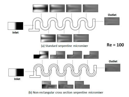
**Figure 6.** Transversal concentration distribution at various positions along the channel for (**a**) a standard serpentine micromixer and (**b**) a serpentine micromixer with a non-rectangular cross-section (Re = 100).
