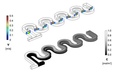
**Figure 4.** Velocity magnitude (cross-sectional maps) (**top**) and concentration distribution (surface map) (**bottom**) along the channel of a non-rectangular cross-section serpentine micromixer ( $R_{in} = W/2 = 100 \mu m$ , and Re = 20).
