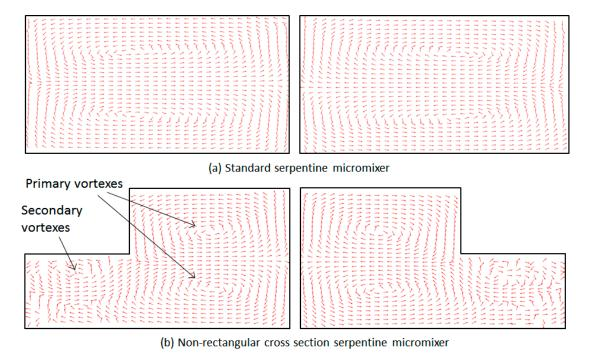
**Figure 8.** Arrow plots of the velocity field for the two mixers design: (a) a standard micromixer and (b) a non-rectangular cross-section micromixer. Both sets of data are collected for the 2nd mixing cycle at Re = 20. The left plots are for data collected at the midpoint of the first leg of the mixing cycle, while the right images are the corresponding plots for the second leg of the mixing cycle.
