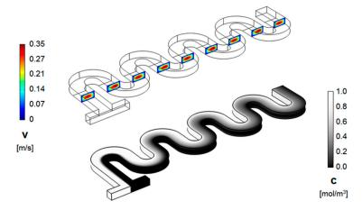
**Figure 3.** Velocity magnitude (cross-sectional maps) (**top**) and concentration distribution (surface map) (**bottom**) along the channel of a standard serpentine micromixer ( $R_{in} = W/2 = 100 \mu m$ , and Re = 20).
