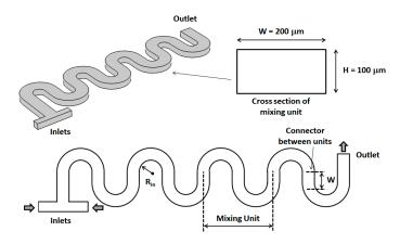
**Figure 1.** 3D and top views of the standard serpentine micromixer with a rectangular cross-section defined by  $W = 200 \mu m$  and  $H = 100 \mu m$ .
