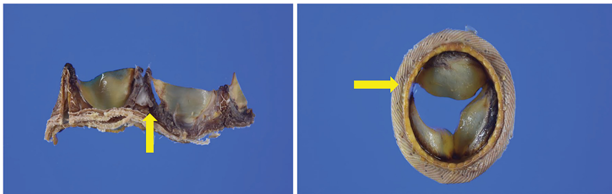
Figure 1. Representative photographs of explanted Trifecta valves. Arrows indicate a tear around the commissure post.
