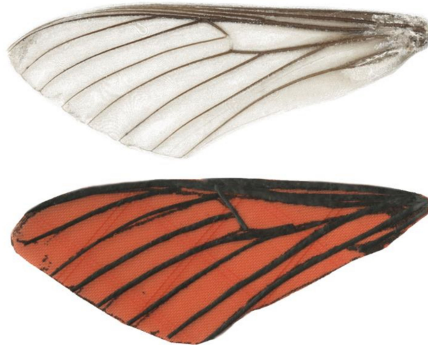
Figure 1. (top) 2D scan of natural forewing excised from Manduca sexta (bottom). Artificial forewing used in this study. These manufactured wings have an approximate wing length of 50 mm, chord length of 20 mm, and mass of 40 mg. Their membrane is made of Icarex™ ripstop polyester, and their venation structure is constructed of Gurit prepreg unidirectional carbon fiber [2].
