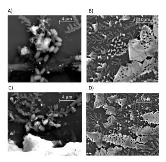
**Figure 7.** SEM microscopy images of quaternized PDMAEMA nanolayers after 24 h of exposure to bacteria with visible bacterial cells: (**A**,**B**) star nanolayers (sample QSG4, Table 5); (**C**,**D**) linear nanolayers (sample QSL4, Table 5).
