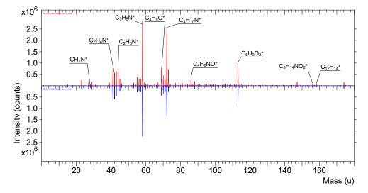
**Figure 4.** Mass spectra of the SG3 (red) and SL3 (blue) samples collected in positive polarity. The intensity scale of mass spectra of the SL3 sample is reversed for easier comparison of the intensities of a particular ion.
