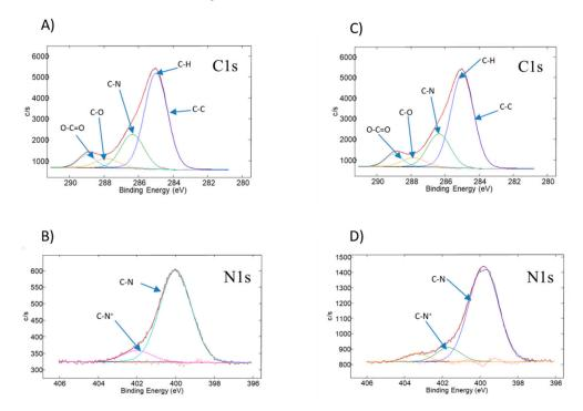
**Figure 3.** The deconvoluted lines of XPS spectra: (**A**) the C 1s core level of the star polymer layer, (**B**) the N 1s core level of the star polymer layer (sample SG3, Table 2), (**C**) the C 1s core level of the linear polymer layer, and (**D**) the N 1s core level of the linear polymer layer (sample SL3, Table 2).
