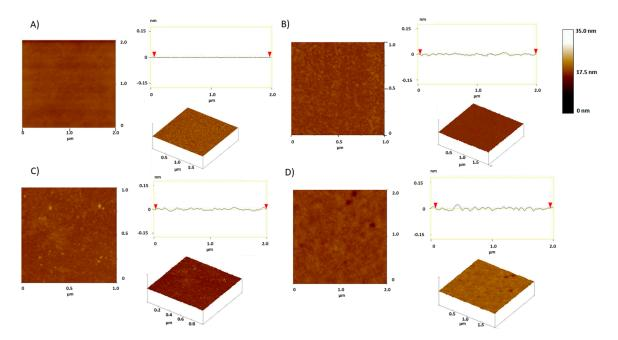
**Figure 1.** Atomic force microscopy images: **(A)** bare wafer with -OH group, **(B)** wafer with benzophenone derivative, **(C)** wafer with immobilized linear PDMAEMA (sample L3, Table 1), and **(D)** wafer with immobilized star PDMAEMA (sample G3, Table 1).
