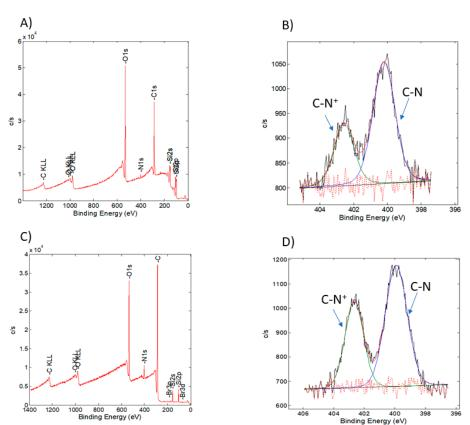
**Figure 6.** XPS spectra of the QPDMAEMA nanolayers: (**A**) survey spectra and (**B**) the N 1s core level of the linear QPDMAEMA nanolayer (sample QSL4, Table 4); (**C**) survey spectra and (**D**) the N 1s core level of the star QPDMAEMA nanolayer (samples QSG4, Table 4).
