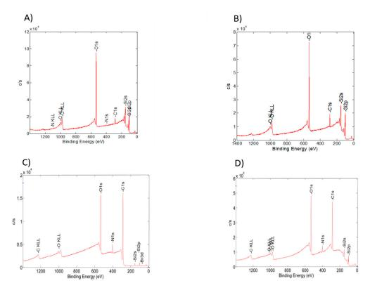
**Figure 2.** XPS survey spectra of (**A**) the OH terminated surface, (**B**) the BPH terminated surface, (**C**) the star polymer layer (SG3, Table 2), and (**D**) the linear polymer layer (SL3, Table 2).
