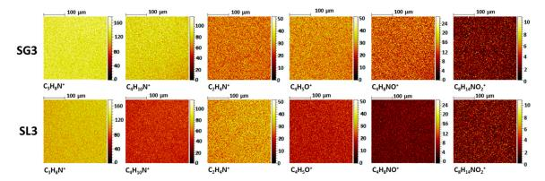
**Figure 5.** Distribution maps of selected ions obtained from the  $300 \times 300 \, \mu m$  areas for the SG3 (first line) and SL3 nanolayers (second line). The intensity scale of distribution maps was unified within a particular ion.
