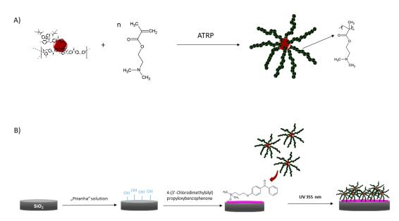
**Scheme 1.** Preparation of the star polymer layers. **(A)** Synthesis of star polymers via the "core-first" method. **(B)** Immobilization of the polymer on the solid support. ATRP, atom transfer radical polymerization.
