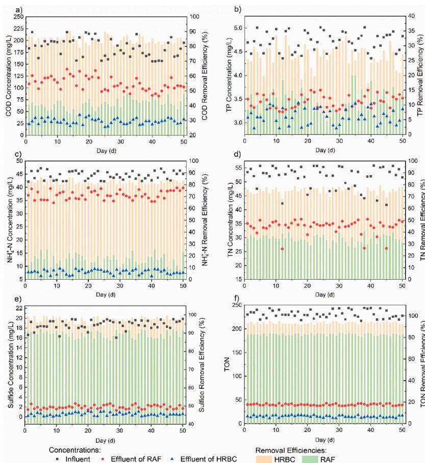
**Fig. 5.** The performance of RAF-HRBC during the 50-day operation. The removal of COD (a), TP (b),  $\text{NH}_4^+$ -N (c), TN (d), and the deodorization efficiency (e), (f).
