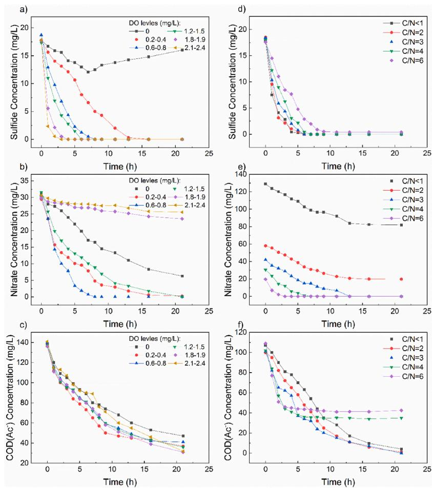
Fig. 3. C–N–S removal time courses under different DO and C/N levels.
