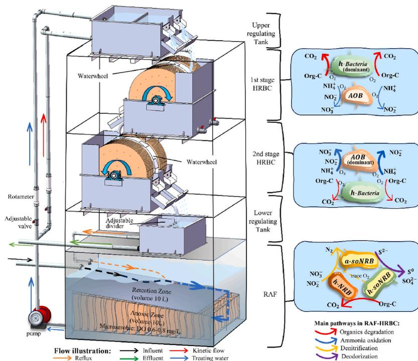
Fig. 1. Diagram of RAF-HRBC scheme and degradation pathways in the system.
