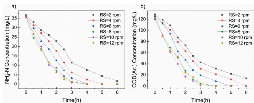
Fig. 4. The time evolution of  $\text{NH}_4^+\text{-N}$  and COD removal under different RSs.
