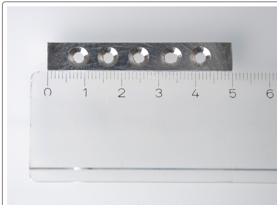
Figure 1 Picture of a non-corroded plate. The plate consists of ZEK100 and has a dimension of 50 mm \times 8 mm \times 1 mm. In every plate five screw holes were drilled and counterbored with an inner diameter of 3 mm on the bone-side and a counterbore diameter of 5 mm.
