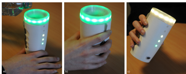
FIGURE 1. The SyMPATHy cup: (a) grasped on the handprint; (b) being filled with water; and (c) tilted during manipulation.
