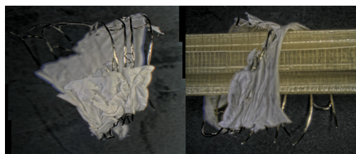
Fig. 3. iCast stent fracture pattern. Unpredictable fracture pattern of iCast stents (left) with occasional development of oval-shaped configuration prior to complete fracture (right).
